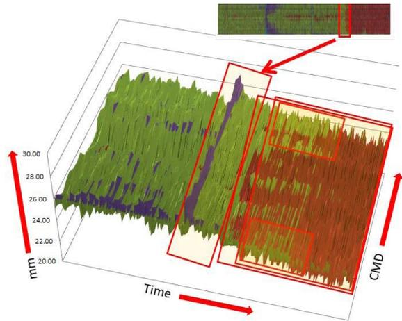
Fig. 3 - Nip width vs. roll cover & felt changes
