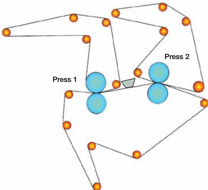
*“This increased compressing of the felt will reduce the effectiveness of the felt to carry water away from the nip, ultimately reducing the felt life in the machine which will increase the costs of operating the machine.”*
