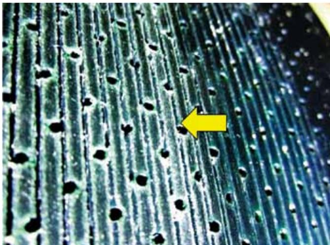
**Non-uniform press load caused premature wear.**
