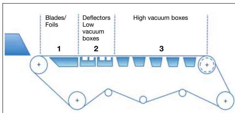
Figure 4. Dewatering elements on a Fourdrinier paper machine.
