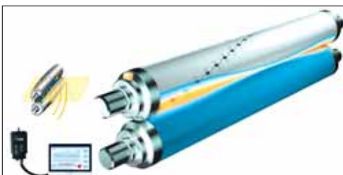
Figure 4. Electronic sensors monitor nip conditions in real time.
